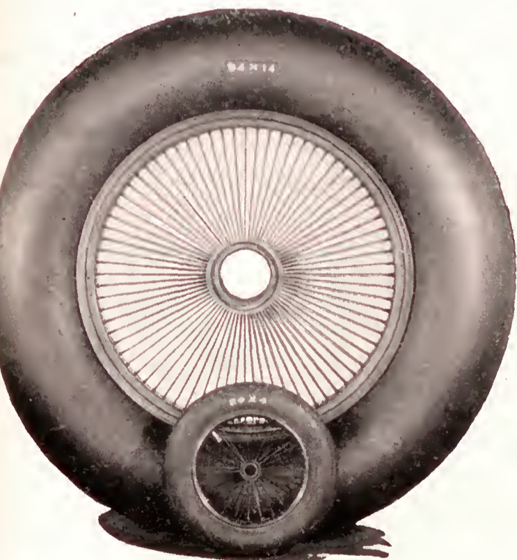
This picture shows the giant and the pigmy of airplane wheels. As shown on the plane above, all airplane wheels are "streamlined" with canvas liners to cut down wind resistance--hence the disc appearance.
